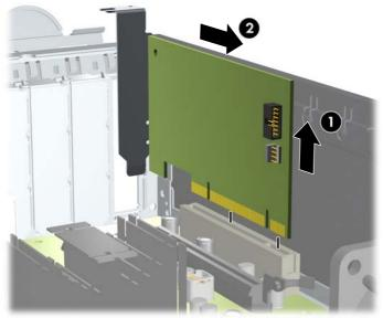
Figure 6-19 Removing a Standard PCI Expansion Card
